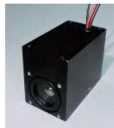
The M2012 photon counting detector is a high sensitivity photon technology detector which is composed of head-on photomultiplier, high voltage power supply module and comparative forming circuit. Before the product leaves the factory parameter point has been preset as the optimal value, the user only needs to switch on the power supply, the output terminal and the counter can be used.
