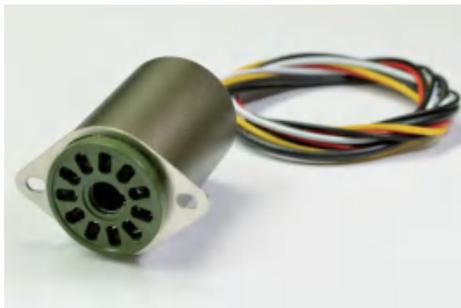
The high voltage tube socket uses  $\pm 15V$  voltage input,  $50k\Omega$  potentiometer or  $0-5V$  voltage control, easy to use and convenient. The main feature is that the built-in voltage divider adopts active voltage divider design, which can make the photomultiplier tube have high DC output linearity. This product is suitable for side-on photomultiplier tube, which has the advantages of high linear DC output, wide output voltage range, fast response speed, low ripple noise and so on.
