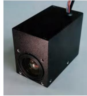
M2021 light detector is composed of head-on photomultiplier tube, power supply circuit and amplifier circuit. The current signal output by the photomultiplier tube is changed into a voltage output signal after I-V amplification. The gain of the light detector can be controlled by resistance adjustment or voltage adjustment.
