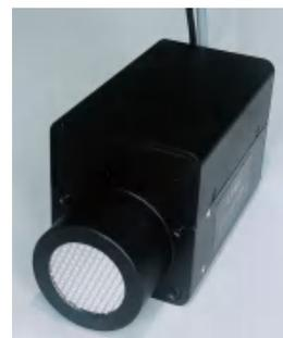
M3013  $\beta$  detector can measure low energy  $\beta$  ray, because of its excellent anti-interference ability, can be widely used in environmental detection, precision measurement, scientific research and other fields. The M3013  $\beta$  detector is mainly composed of end window photomultiplier, high voltage power supply module, signal forming circuit, scintillator and so on.
